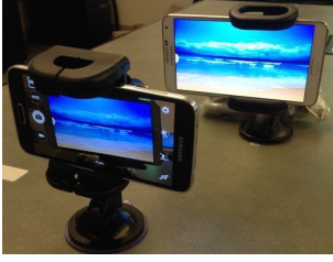
Figure 6: Experimental setup with Samsung Note 3 (right) as the transmitter and Samsung S5 as the receiver (left).
