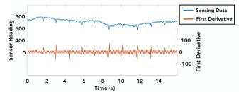
Figure 6: Time series of the harvested power of a photodiode. The photodiode is carried by a walking user, who swipes a finger above the photodiode nine times.
