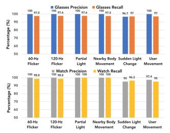
Figure 13: Accuracy of gesture recognition under ambient light fluctuations.
