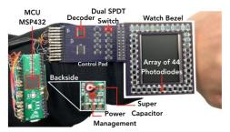
Figure 8: Integrating the prototype with a smart watch.
