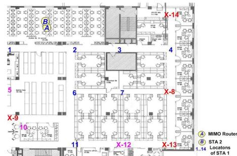
Figure 3: Testing positions. At red points STA1 can not connect with AP. At pink ones connection is unstable. Blue points are normal.
