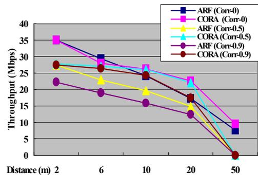
Figure 9: Throughput of single flow under different correlated channels
