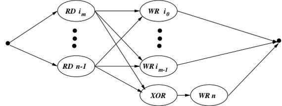
Figure 4: DAG 4, Large Write DAG, no failure
