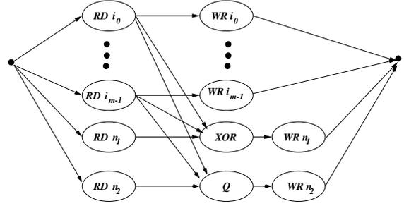
Figure 10: RAID Level 6 - Small Write.
