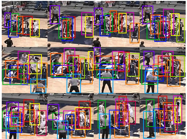
Fig. 1: An example of the difficult problem that our interactive system addresses. The red boxed player becomes totally occluded while many players quickly change pose from standing to a prone position. The referees commonly enter and leave the scene. The camera is not stationary. The ball exists in the pile of people, but even a state-of-the-art vision algorithm is unable to determine its position.
