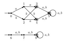
Here we have modified the first automaton by making states 3, 4 accept states instead of 1, 2. Now states 3, 4, 5 are equivalent and can be collapsed. These become state 8 of the second automaton. The set accepted is the set of all strings of length at least two.  $\hfill \Box$
