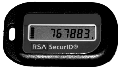
Figure 3.1: An RSA SecurID authentication token.
