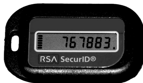
Figure 3.1: An RSA SecurID authentication token.
