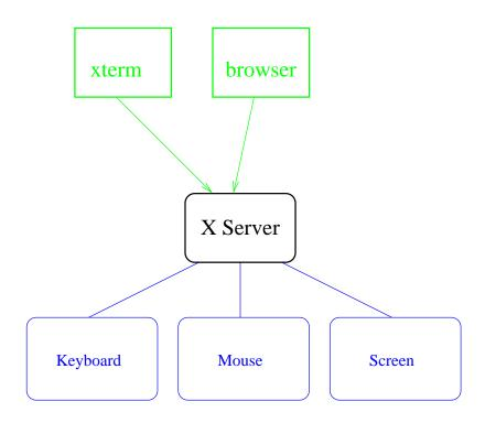
The X server controls the keyboard, screen, and mouse. X applications contact the server — perhaps over the network — to interact with the user.
