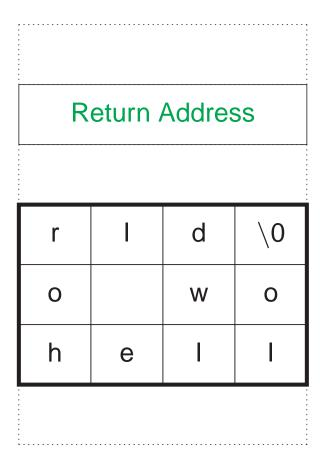
When a function is called, the return address is stored on the stack. Lower in memory, all local variables are stored.
