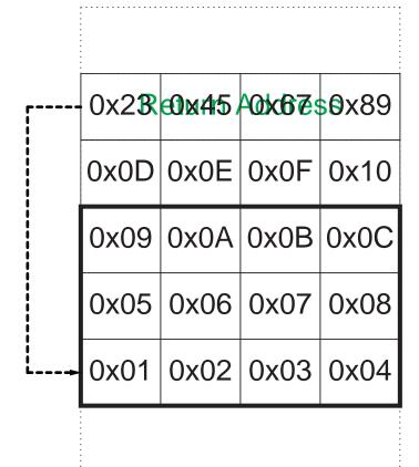
Put code in the early part of the buffer, then change the return address to point to it. When the function exits, the injected code is executed.
