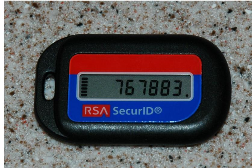
A SecurID token on two successive time cycles. The bars on the left of the second picture indicate how many 10-second ticks remain before the display changes, in this case about a minute. In essence, the display shows  $H_k(T)$ , where  $T$  is the time and  $H_k$  is a keyed hash function.
