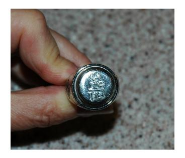
This ring has a Java interpreter, a crypto chip, and certificate-processing code. Google and others are pushing NFC rings.
