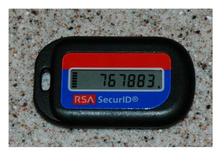
A SecurID token on two successive time cycles. The bars on the left of the second picture indicate how many 10-second ticks remain before the display changes, in this case about a minute. In essence, the display shows  $H_k(T)$ , where T is the time and  $H_k$  is a keyed hash function.
