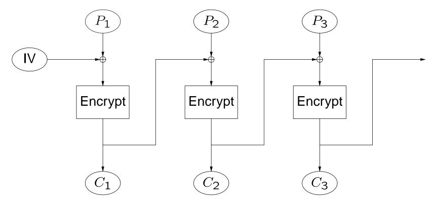
$\{P_i \oplus C_{i-1}\}_k \to C_i$  $\{C_i\}_{k-1} \oplus C_{i-1} \to P_i$
