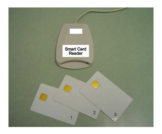
These cards use contacts for power and I/O. Other types use inductive coupling or radio.
