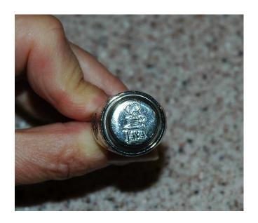
This ring has a Java interpreter, a crypto chip, and certificate-processing code.
