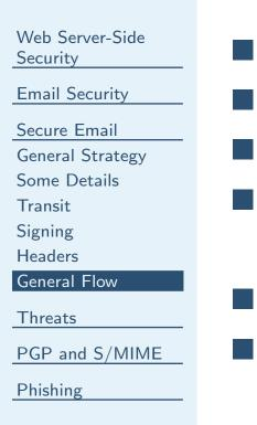
Collect input message Put in canonical form Encrypt and sign, or sign and encrypt Add metadata: encrypted traffic key, your certificate, algorithm identifiers, etc. Convert to transit form Embed in email message
