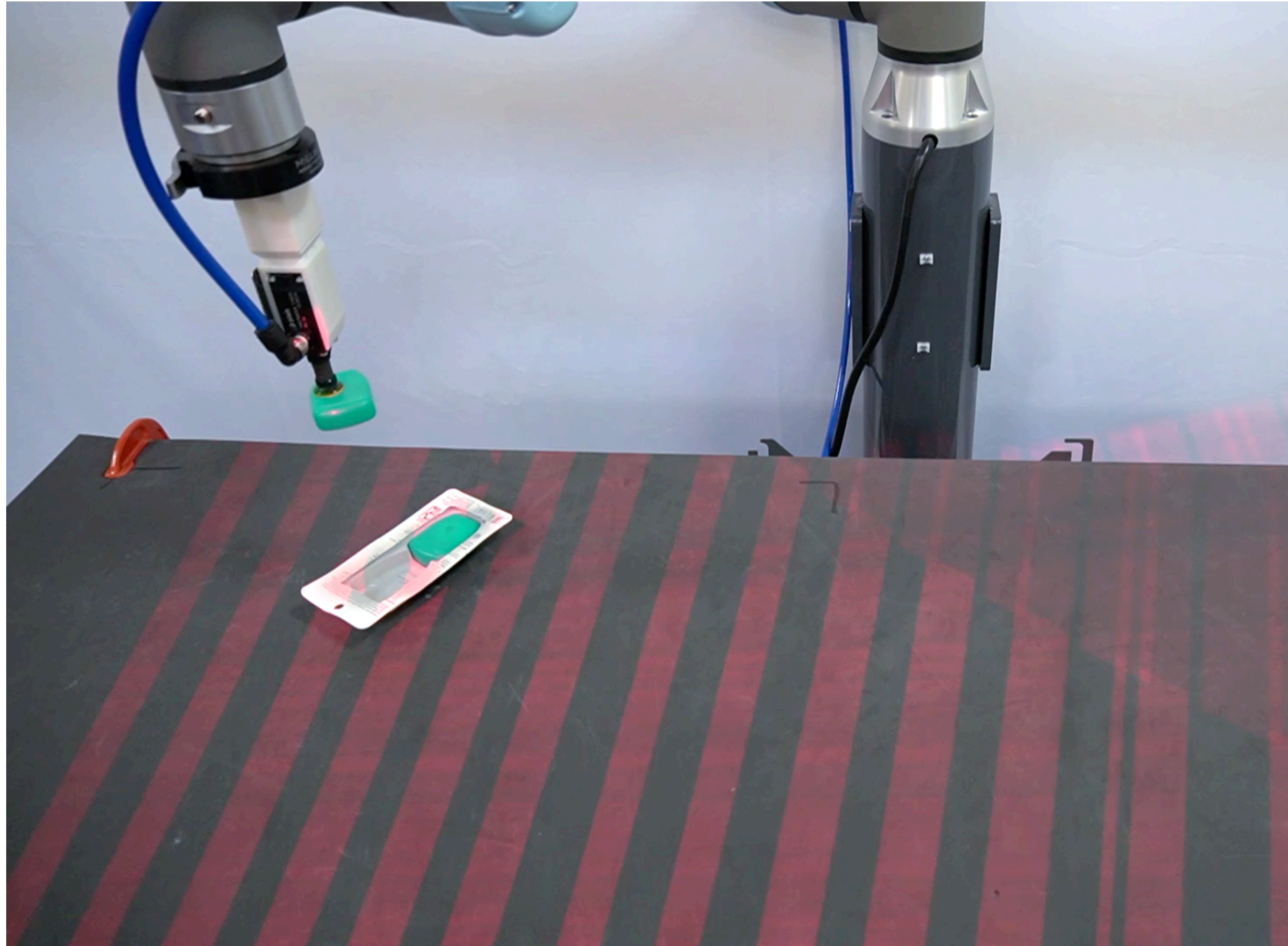
Top-down pick and place with 2D rotation
