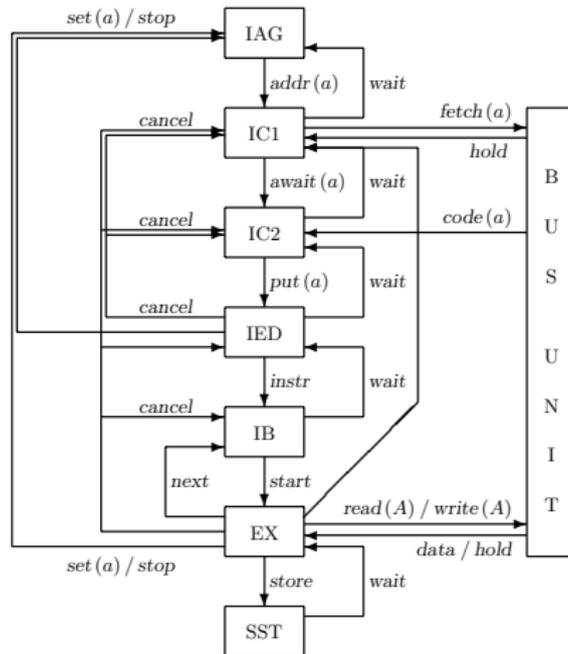
Motorola Coldfire pipeline from Ferdinand et al., Reliable and precise WCET determination for a real-life processor, EMSOFT 2001
