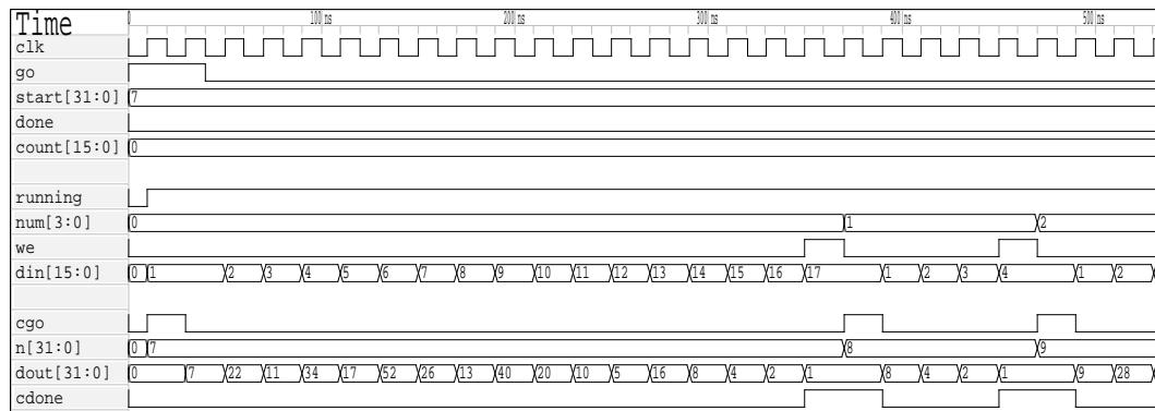
The *go* input switches *running* to true; loads *n* with the value on *start*; resets *num*, the RAM address, to 0; sets *din*, the iteration count, to 1; and pulses *cgo* high for a cycle to start the Collatz iterator module.
