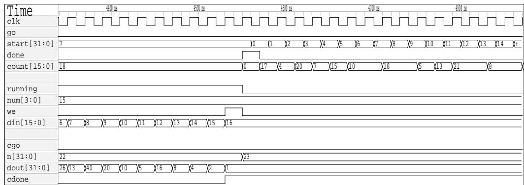
After *we* is asserted for the highest RAM address (15, set by *RAM\_WORDS*), *running* turns off and *done* pulses once. This tells the testbench to feed 0, 1, 2, ... into *start* and the number of iterations for each value is read out on *count*. For example, *start* = 0 produces a 17 on *count*, corresponding to  $n = 7$ , and *start* = 11 produces a 21, corresponding to  $n = 7 + 11 = 18$ .
