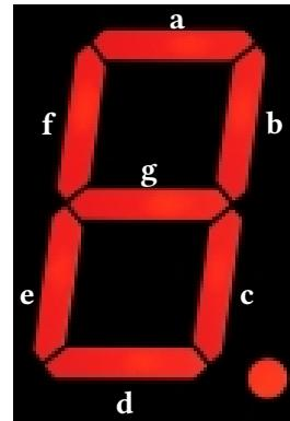
Implement the body of the seven-segment decoder module in *hex7seg.sv*. We have provided a Verilator testbench to test your implementation. Make sure Verilator is installed and compile and run the simulation:
