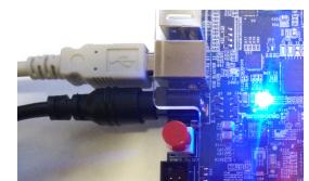
Once your project is compiled, download the *.sof* file to the DE1-SoC board by running `make` program. A variety of things can go wrong. If you get “Error (213013): Programming hardware cable not detected,” check your board’s power and USB connection to your workstation.
