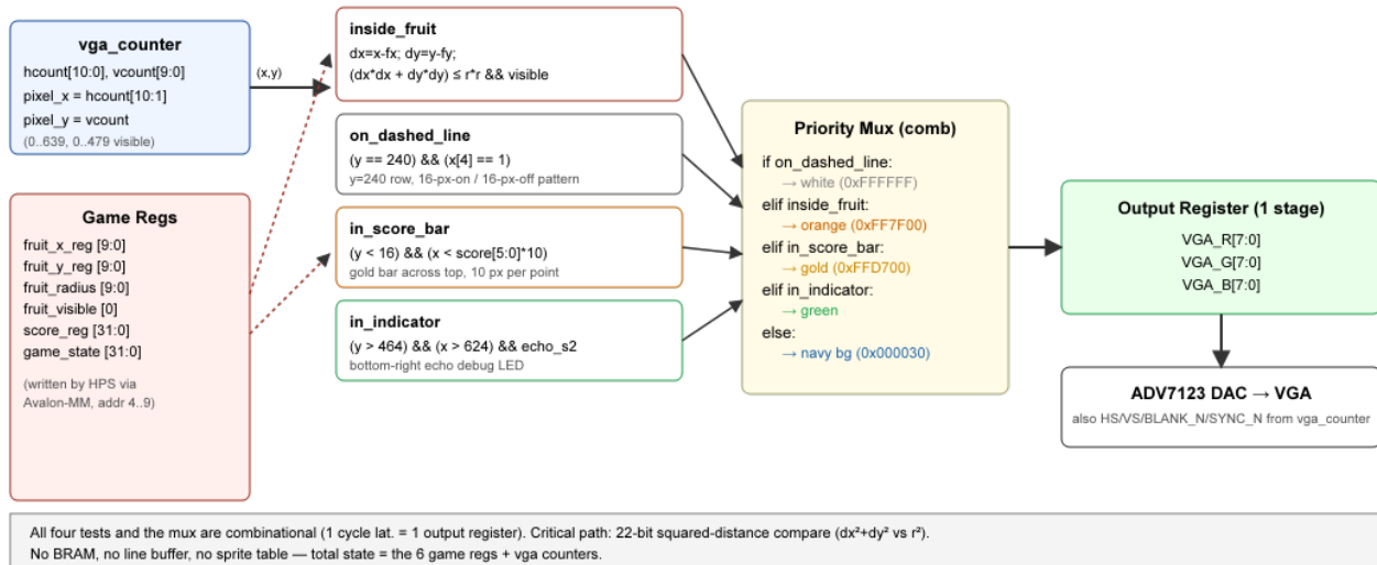
Figure 3: Combinational pixel renderer.
