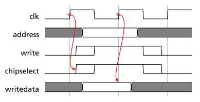
Bus cycle starts on rising clock edge Data available by next rising edge Peripheral may be synchronous, but must be fast Basic Async. Agent Write w/ 1 Wait State
