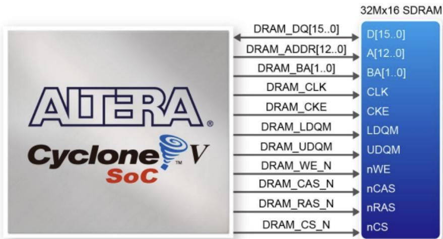
Fig 11: FPGA-SDRAM interface
