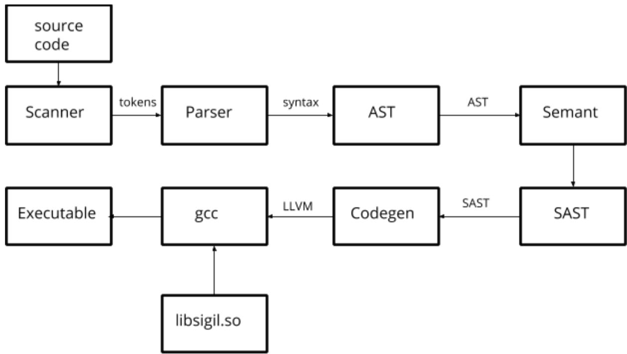
The frontend of the ZEN to LLVM compiler `zen.ml` calls each of the above components in order. When a user executes “`make zen.native`” the entire compiler sequence is run. First, ZEN source code is passed through the scanner and parser, generating the AST. The AST is passed through the semantic checker, which
