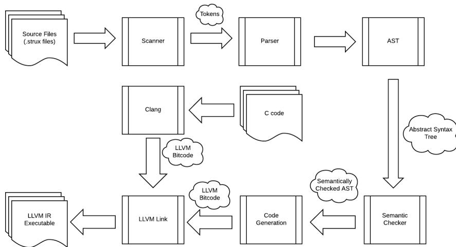
The architectural design of Strux is very similar to that of MicroC, with the exception of Strux having additional C modules that are linked with codegen LLVM bitcode to form the LLVM IR.
