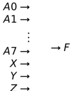
Here,  $A0$  through  $A7$  are the eight inputs, and  $X$ ,  $Y$ , and  $Z$  are the three selects.  $X$  is the most significant bit, selecting between, e.g.,  $A0$  and  $A4$ .
