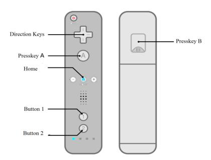
Wiimote input outperform traditional Keyboard and Mouse input. The game controlled by Wii makes it possible for a wireless remote input, which gives user a more convenient, better and more comfortable feeling in operation. All the game process can be implemented with only one hand! Wiimote brings more fun. In order deal with basic control in the game, we will use direction keys, Press-key A and B, as well as Button 1 and 2. The four direction keys are responsible for movement along
