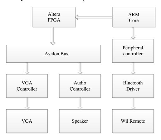
As shown in the block diagram, we have Altera SOC FPGA with Arm embedded cores as key part and 4 peripheral components: SRAM controller, VGA controller, Audio Controller and Peripheral controller for Wii mote. The Avalon bus is the communication bus between different components.
