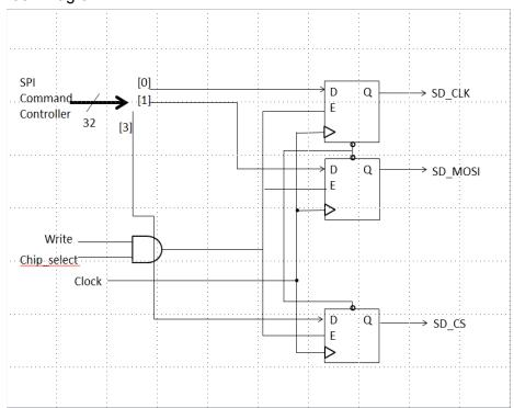
SPI Command Controller sends the appropriate initialization commands to the SD card from Nios II.
