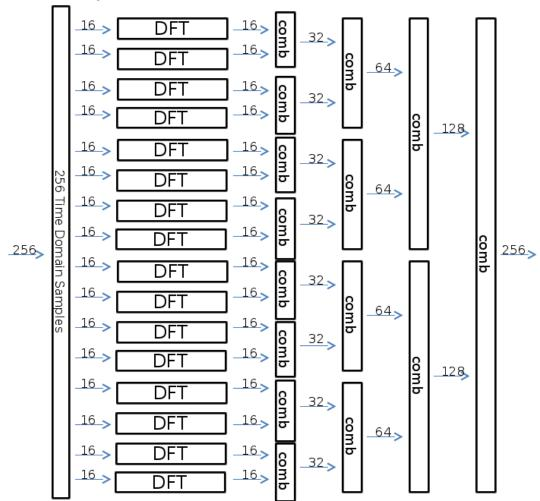
This is a radix-16 DFT, so we split the inputs into 16 different parts and perform a DFT on each group according to the equation
