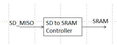
SD\_MISO comes from the SD Card. Normally this goes into the SPI interface however in this case we are writing it straight to SRAM instead.
