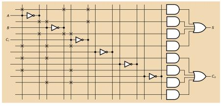
$$S = A \oplus B \oplus C_i = A\overline{B}\overline{C_i} + \overline{A}B\overline{C_i} + \overline{A}\overline{B}C_i + ABC_i$$
