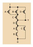
(b) Draw the schematic for a static CMOS gate that implements  $Y = \overline{(AB + C)D}$
