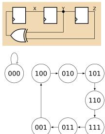
2. (15 pts.) The 1965 Ford Thunderbird had sequential turn signals that would light sequentially. Design an FSM that implements such signals.
