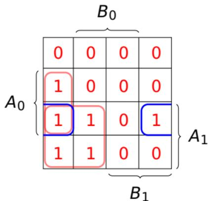
$$A_1 \overline{B_1} + A_0 \overline{B_0} \overline{B_1} + A_0 A_1 \overline{B_0}$$
