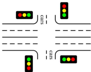
This controls a traffic light at the intersection of a busy highway and a farm road. Normally, the highway light is green but if a sensor detects a car on the farm road, the highway light turns yellow then red. The farm road light then turns green until there are no cars or after a long timeout.
