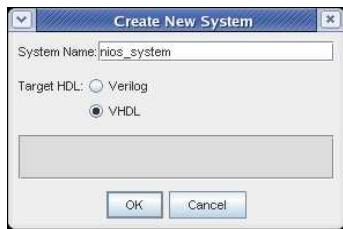
Figure 3: Naming a new system in SOPC Builder
