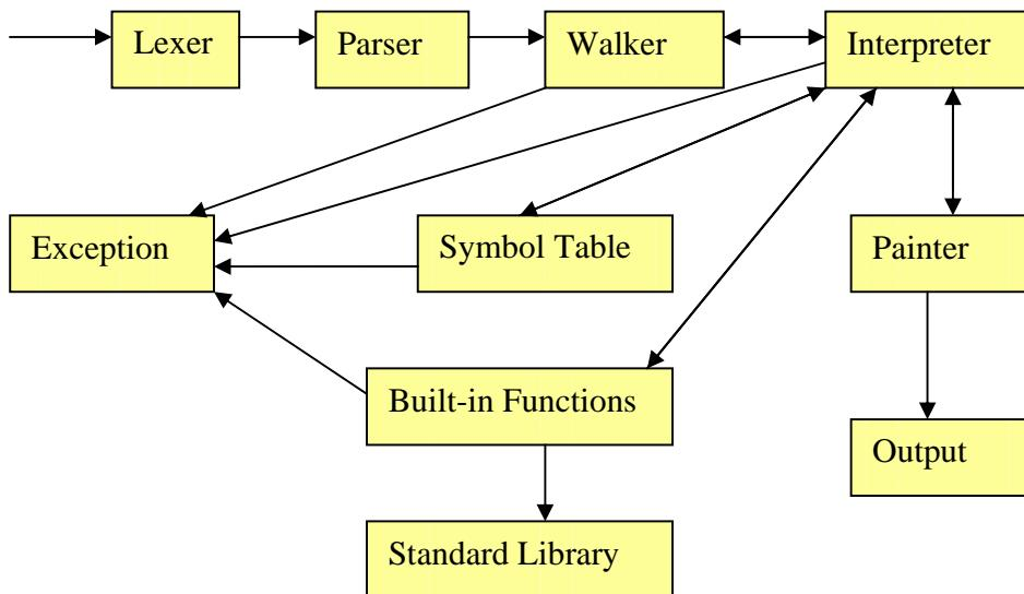
The lexer, parser and tree walker are implemented by Antlr. The lexer and parser are implemented in Antlr file grammar.g, and the tree walker is implemented in Antlr file walker.g. Source file walker.g contains short actions calling the methods in the class Interpreter.
