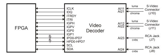
The FPGA pins connect to the video decoder as shown below:
