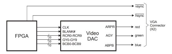
The pin assignments for the connection of the FPGA to the VGA circuitry are shown below.
