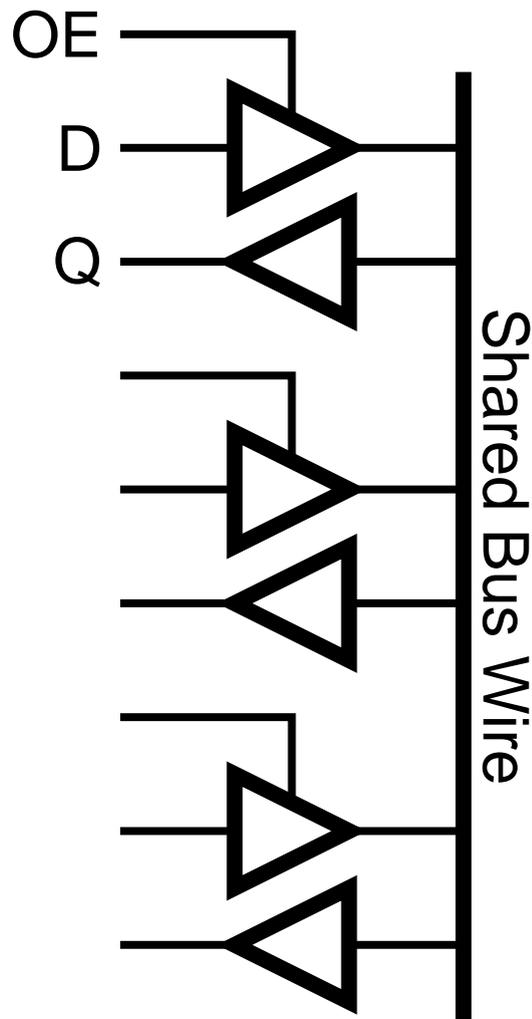
Basic trick is to use a “tri-state” driver than can choose to not drive a wire.
