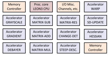
ESP instance for WAMI (Wide-Area Motion Imagery) rapid integration and prototyping
