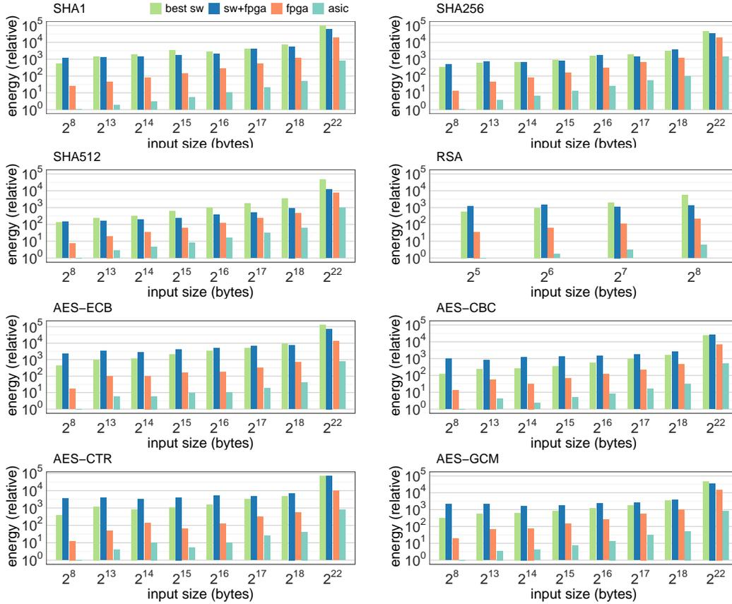
Fig. 6: The figure reports the energy consumption of performing crypto operations in *Hardroid*. We compare (i) the best software implementation (*best sw*), (ii) our accelerators by considering the software overheads for invoking them (*sw+fpga*), (iii) our FPGA accelerators only (*fpga*), and (iv) our ASIC accelerators only (*asic*). The values are relative to the energy consumed by the ASIC accelerators for the smallest inputs.
