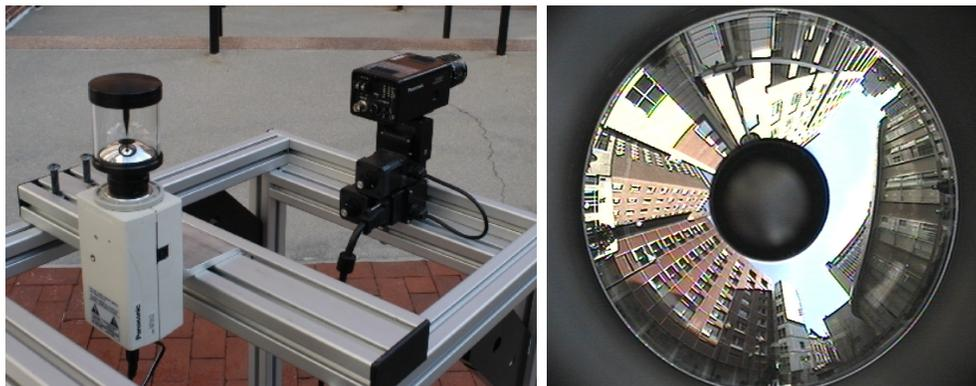
Figure 11: Our robot’s omnicaamera (left) and a typical image from that camera (right).
