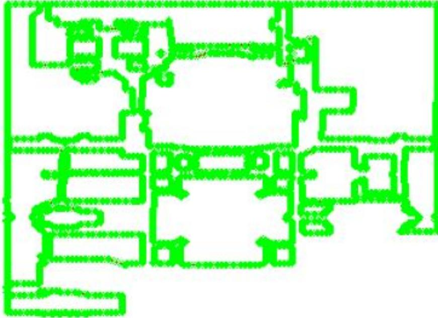
Figure 7: The points that approximate the polygonal obstacles for the generalized Voronoi diagram.
