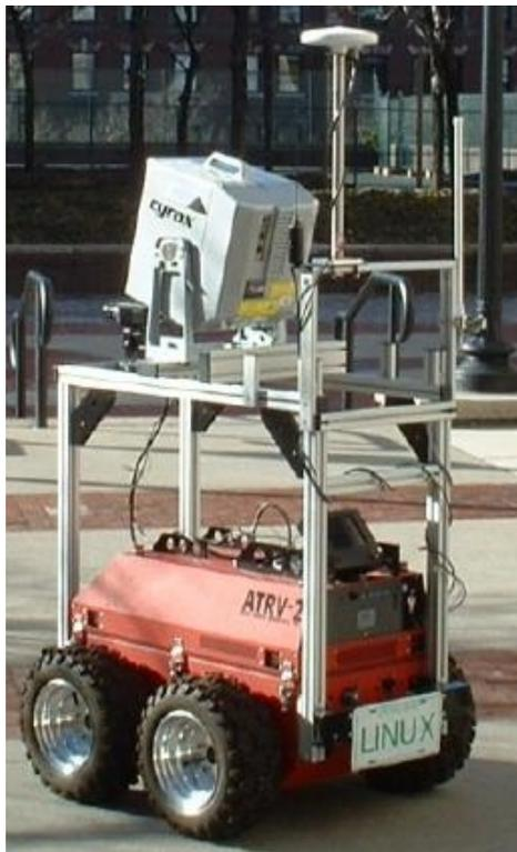
Figure 1: The ATRV-2 Based AVENUE Mobile Robot.
