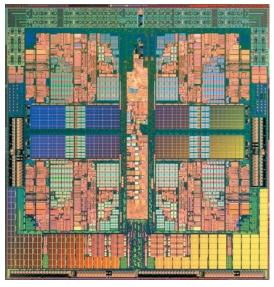
AMD Phenom 9600 Quad-core 2.3 GHz 1.1–1.25 V 95 W 65 nm A desktop machine:
