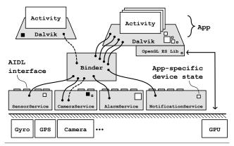
**Figure 2.** Overview of Android system components and their relation to one another through Binder.
