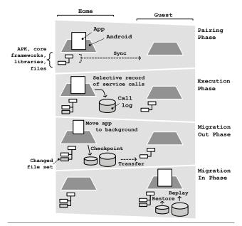
Figure 4. Workflow phases of Flux migration.
