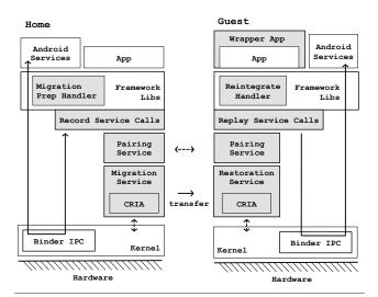
**Figure 3.** Overview of Android components involved in migration. Components added by Flux highlighted in gray.
