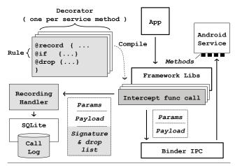
**Figure 5.** Selective Record and its place in the Android system. Flux-specific components highlighted in gray.
