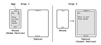
**Figure 1.** Multi-surface support through app migration: swipe to migrate unmodified app between paired devices without cloud support.
