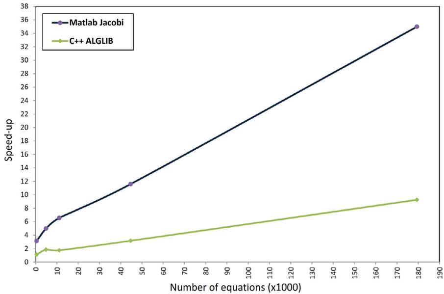
Fig. 13. Speed-up of our 32-bit floating-point Clustered Jacobi hardware over software implementations of MATLAB Jacobi and C++ ALGLIB.
