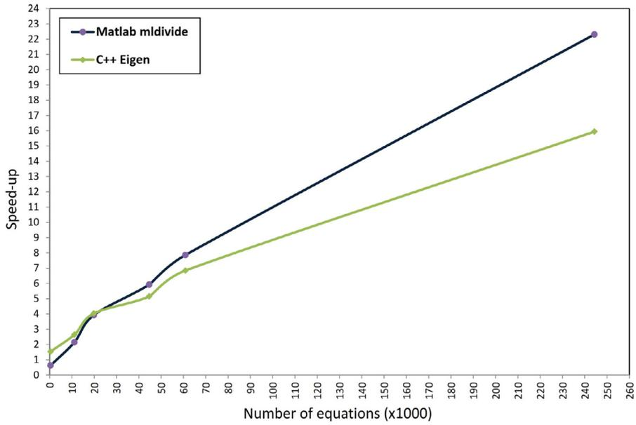
Fig. 12. Speed-up of our 32-bit floating-point Clustered Gaussian hardware over software implementations of MATLAB mldivide and C++ Eigen.
