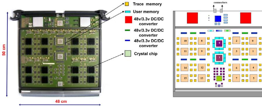
Fig. 10. Construction of Mentor Graphics Veloce 1 Advanced Verification Board (AVB).
