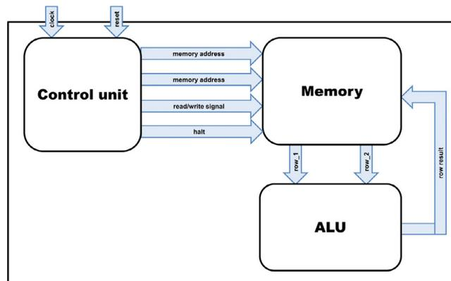
Fig. 4. Block diagram of our Basic Gaussian.
