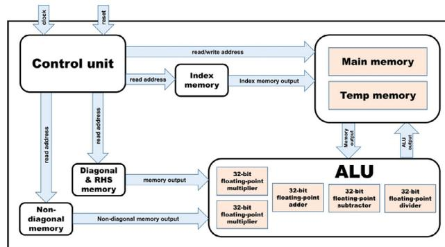
Fig. 7. Block diagram of our Basic Jacobi.
