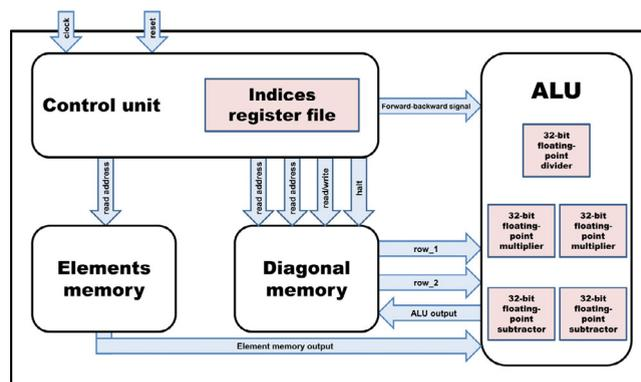
Fig. 5. Block diagram of our Gaussian-using-sparse.
