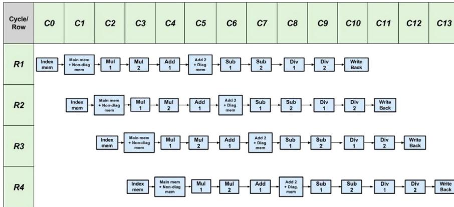
Fig. 8. Multi-clock-cycle diagram for our Pipelined Jacobi. C is the current clock cycle and R is the current row of the coefficients matrix. Each box represents the operation done on a specific row during a specific clock cycle.
