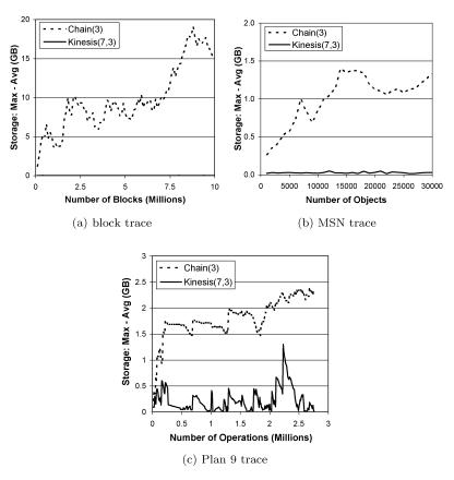
Fig. 4. Storage imbalance: Kinesis(k, 3) vs. Chain(3).
