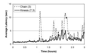
Fig. 11. Latency vs. time: Kinesis(7, 3)'s better load balance leads to lower latencies compared to Chain(3).
