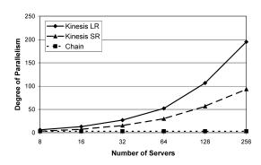
Fig. 9. Kinesis(7, 3) vs. Chain(3): degree of parallelism with varying numbers of servers.
