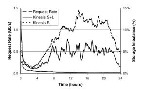
Fig. 8. Storage imbalance vs. time: Kinesis S+L compensates for temporary decreases in storage balance when client activity is low.
