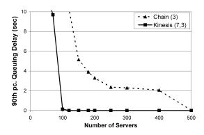
Fig. 5. Kinesis(7,3) vs. Chain(3): 90th-percentile queuing delay for read requests on MSN Video trace, as the number of servers is varied with average read request rate fixed at 2.9GB per second.
