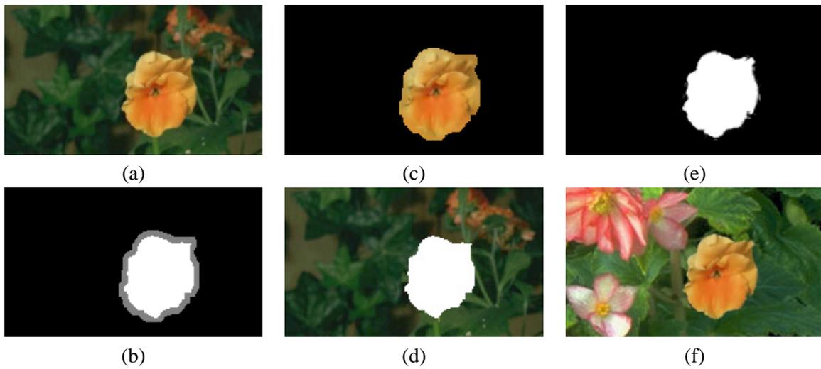
Figure 6.17: Video matting and completion: (a) Frame from input video. (b) Graph cut trimap. (c) Foreground estimation in unknown region. (d) Background completion of unknown region. (e) Alpha matte. (f) Composite.
