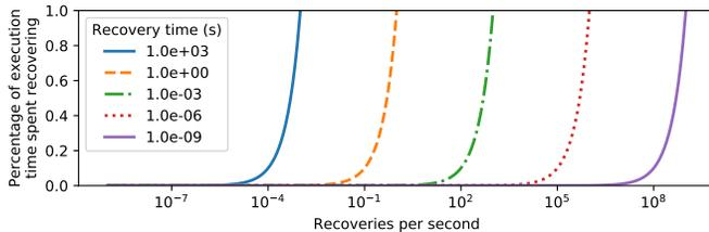
Fig. 1. In order to achieve tolerable overheads, the recovery time must shrink as the rate of recoveries increases.
