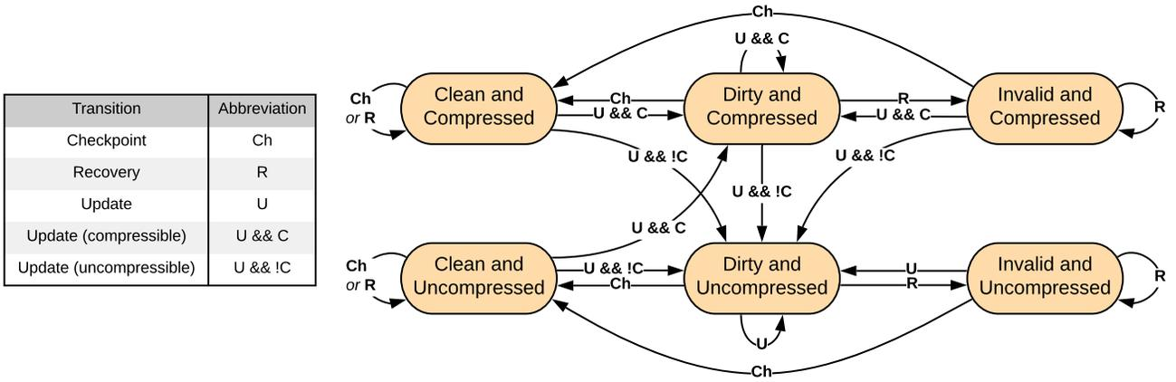
Fig. 2. A state diagram describing a cache line’s transition between states, given various system events.
