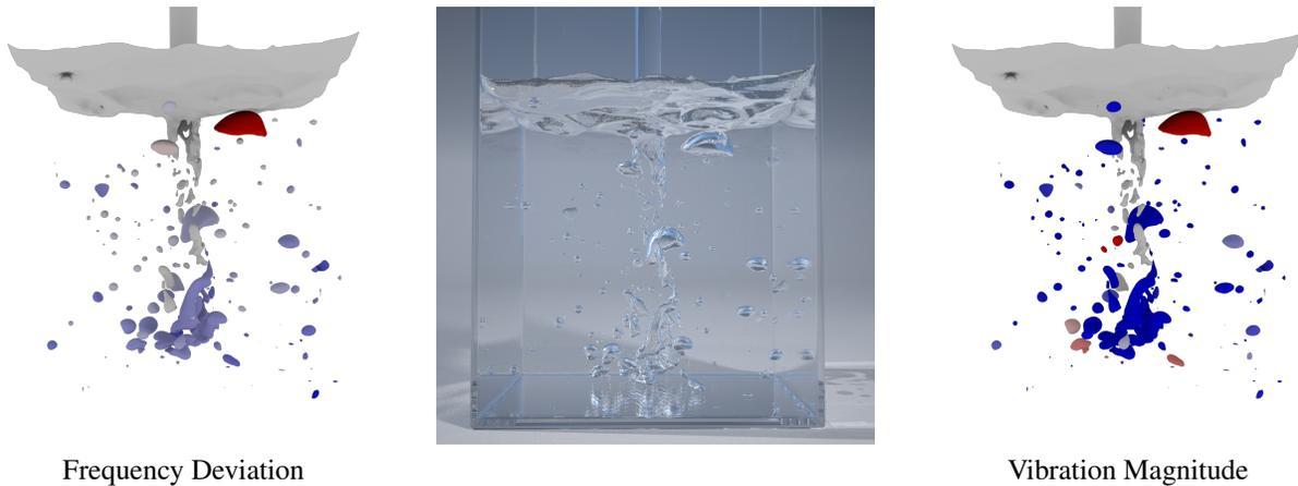
**Figure 1: Complex acoustic bubbles:** Our system is able to capture complex frequency effects due to bubbles' shapes and positions. (Left) Bubbles are colored blue/red if they are lower/higher than the theoretical Minnaert frequency for spherical bubbles, and depicts pitch rise near the surface. (Right) Bubbles are colored (blue/red) based on their (small/large) vibration magnitude.
