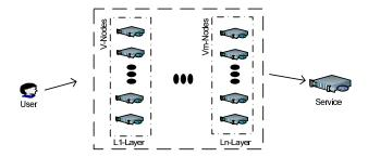
**Fig. 1.** The multilayer overlay network (MON) architecture. Multiple layers of nodes are interposed between the clients and the provided service. The number of layers is configurable at overlay setup, and can be tuned to favor performance over resistance to intrusion by reducing the degree of internal redirection.
