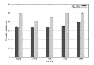
Fig. 7. Average processing time introduced by entry points and core nodes in MON.
