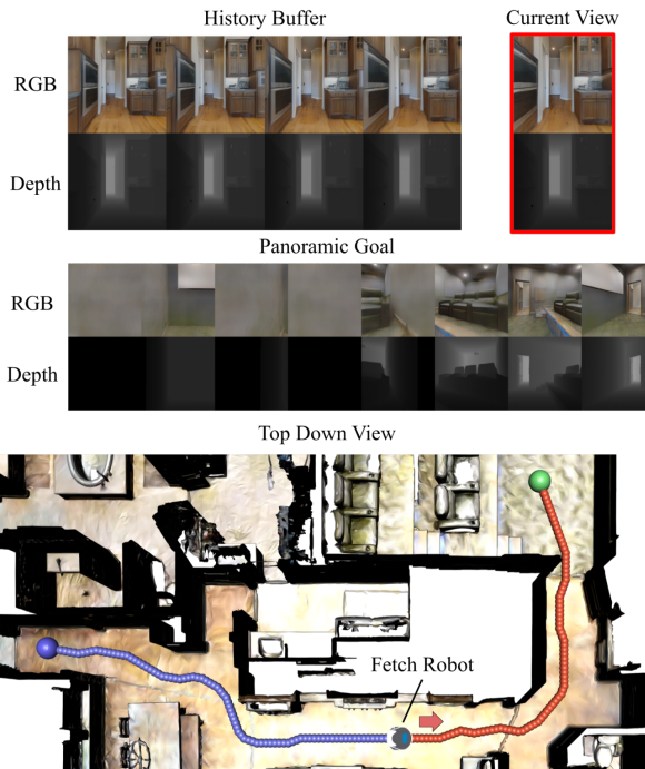
Fig. 1: A successful trajectory executed in house17 from the Matterport3D dataset. The history buffer and current view are the state of the pipeline. The panoramic goal is 8 RGBD images each taken at a 45^\circ turn. The top-down view is the agent moving through the trajectory with the blue sphere as the start position and the green sphere as the goal position. Smaller blue spheres are positions that the agent has been to and the orange spheres are the remaining positions. The images are taken at the current position of the robotic agent.
