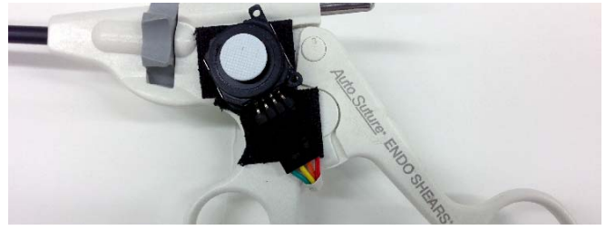
Fig. 4. An image of our prototype SSL Thumbstick. We use a 2-axis button joystick as an add-on to a standard, off-the-self laparoscopic tool to allow the surgeon to perform virtual transformations (translate, rotate and scale) to 3D reconstructed images or Zoom and Pan 2D Images without having to take her/his hands of the laparoscopic tools or change the position of the laparoscopic camera.
