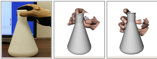
Fig. 4. Grasp planning using human data. Left: grasp executed by human operator. Middle: Low-dimensional approximation of human grasp, also affected by measurement noise. This posture, which only approximates a correct grasp, is used as input for the grasp planner. Right: form-closure grasp found by the planner based on the input data.
