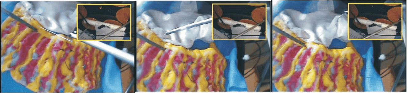
Fig. 4. Prototype I was used in a suturing experiment within a laparoscopic training box. The image provided by the device was sufficiently clear to perform the task without using any additional image sources. The surgeon's assistant was able to adjust the view at the surgeon's request by joystick control of the camera's pan, tilt and translation axes.
