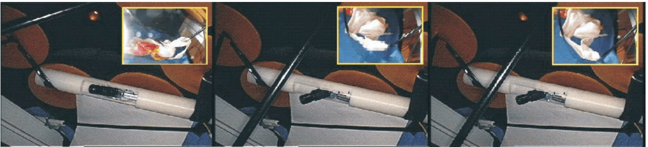
Fig. 5. Prototype I was used in another task that required motions over greater distances and was performed within the training box. Again the assistant was able to keep the activity within the field of view of the camera. This sequence more clearly shows the motions of the camera.
